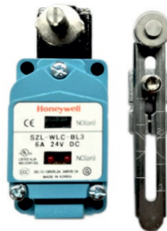
SZL-WLC-B-L3 ADJUSTABLE SIDE ROTARY SPDT - DOUBLE BREAK (1NO 1NC)
