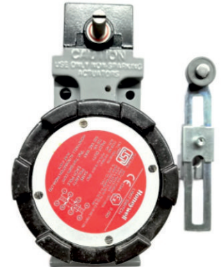
BXINDA4L-2C 3/4" NPT SIDE ROTARY MOMENTARY 2NO/2NC - ADJUSTABLE LEVER
